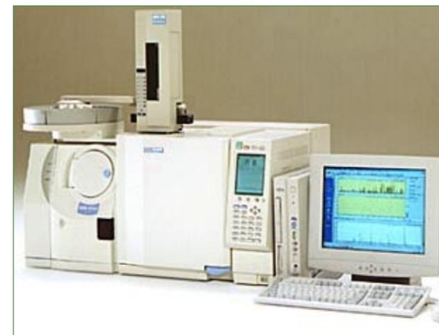
Gas chromatograph-mass spectrometer for faecal sterol measurements
